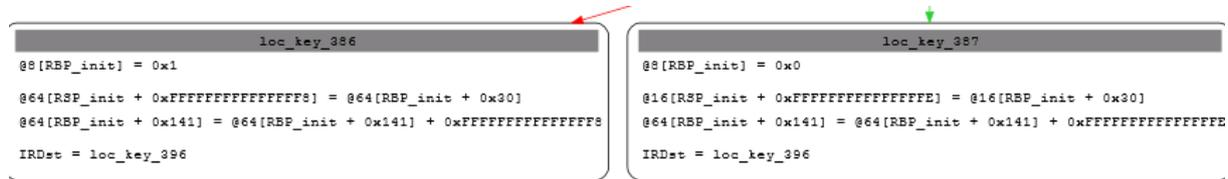
Figure 37. Part of the fourth virtual instruction performing a `PUSH` operation
