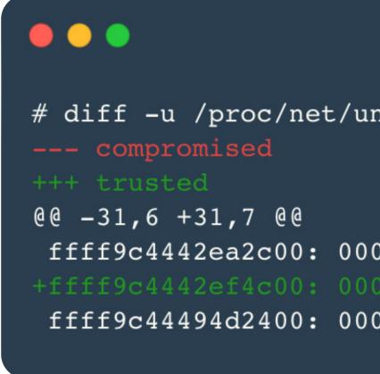
Figure 17. Difference between /proc/net/unix seen under a program compromised with Ebury and one that is not
