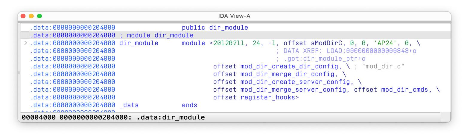
Figure 22. Module information exported by mod\_dir.so as seen in IDA Pro with the proper structure definition
