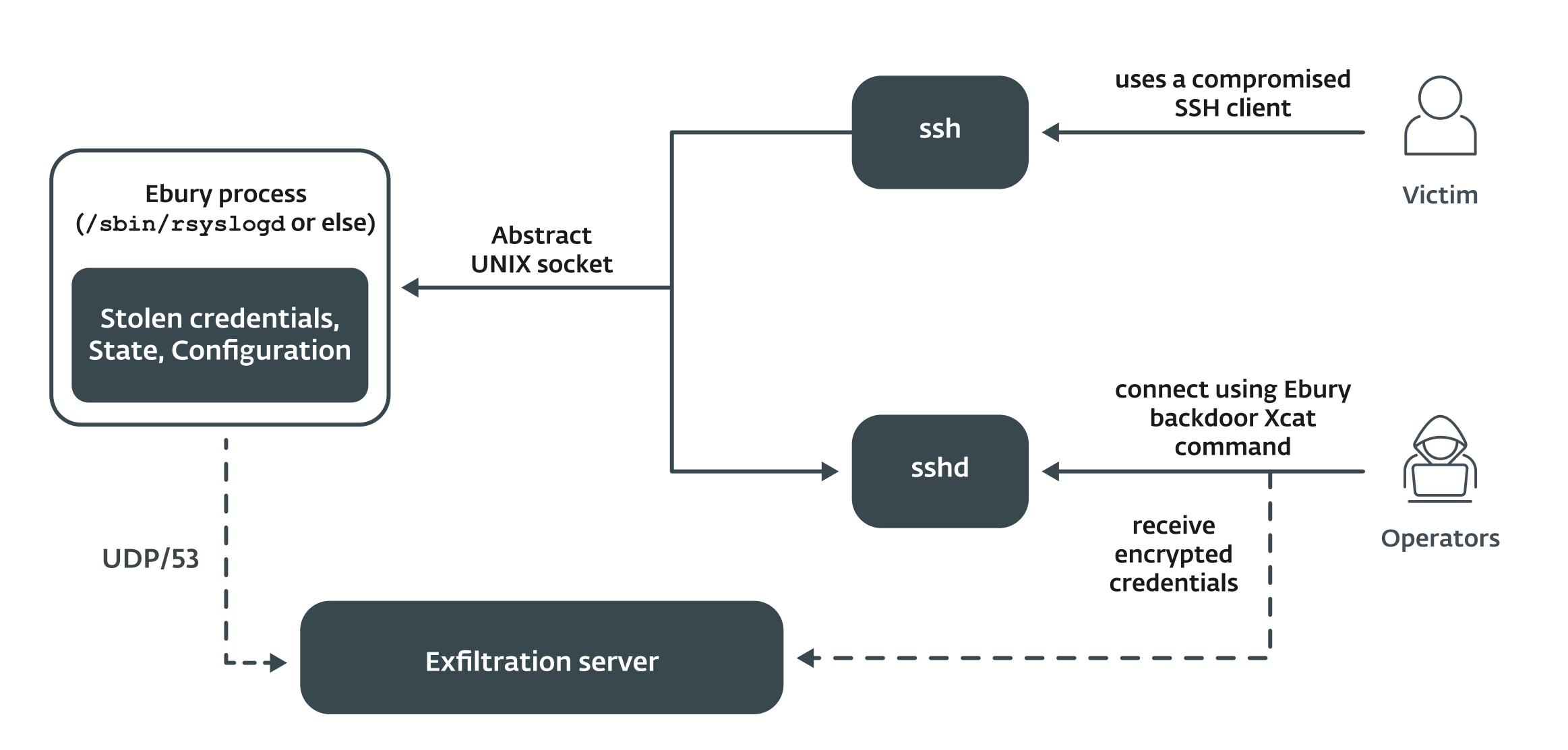
Figure 12. Flow of stolen credentials, from the victim using an Ebury-compromised SSH client to the Ebury process, and later fetched by the operators
