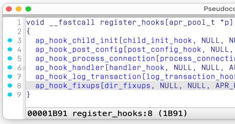
Figure 23. Hex-Rays Decompiler output for HelimodProxy's register\_hooks
