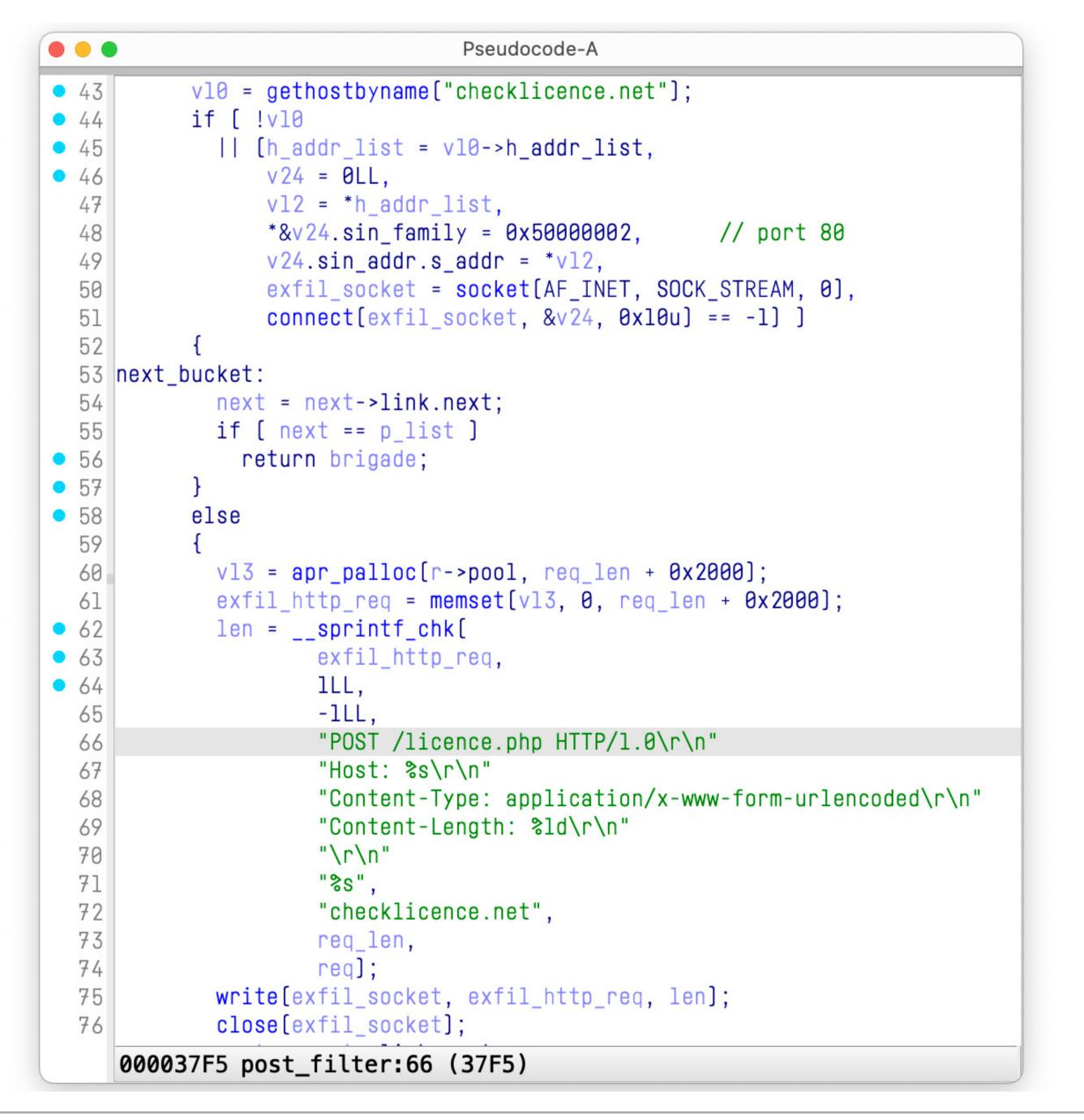
Figure 26. Hex-Rays Decompiler output of HelimodSteal input filter, exfiltrating data using an HTTP request
