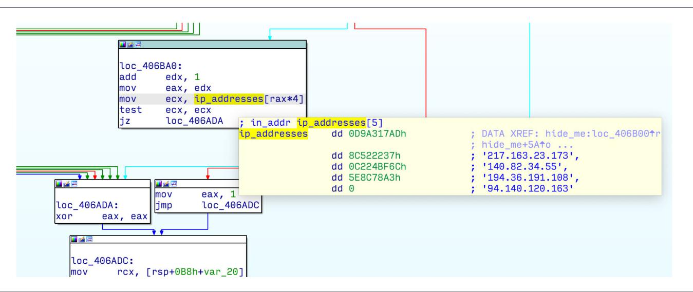
Figure 41. IDA Pro flow graph showing an IP address being compared with the embedded, hardcoded list to determine whether to display it in the command output
