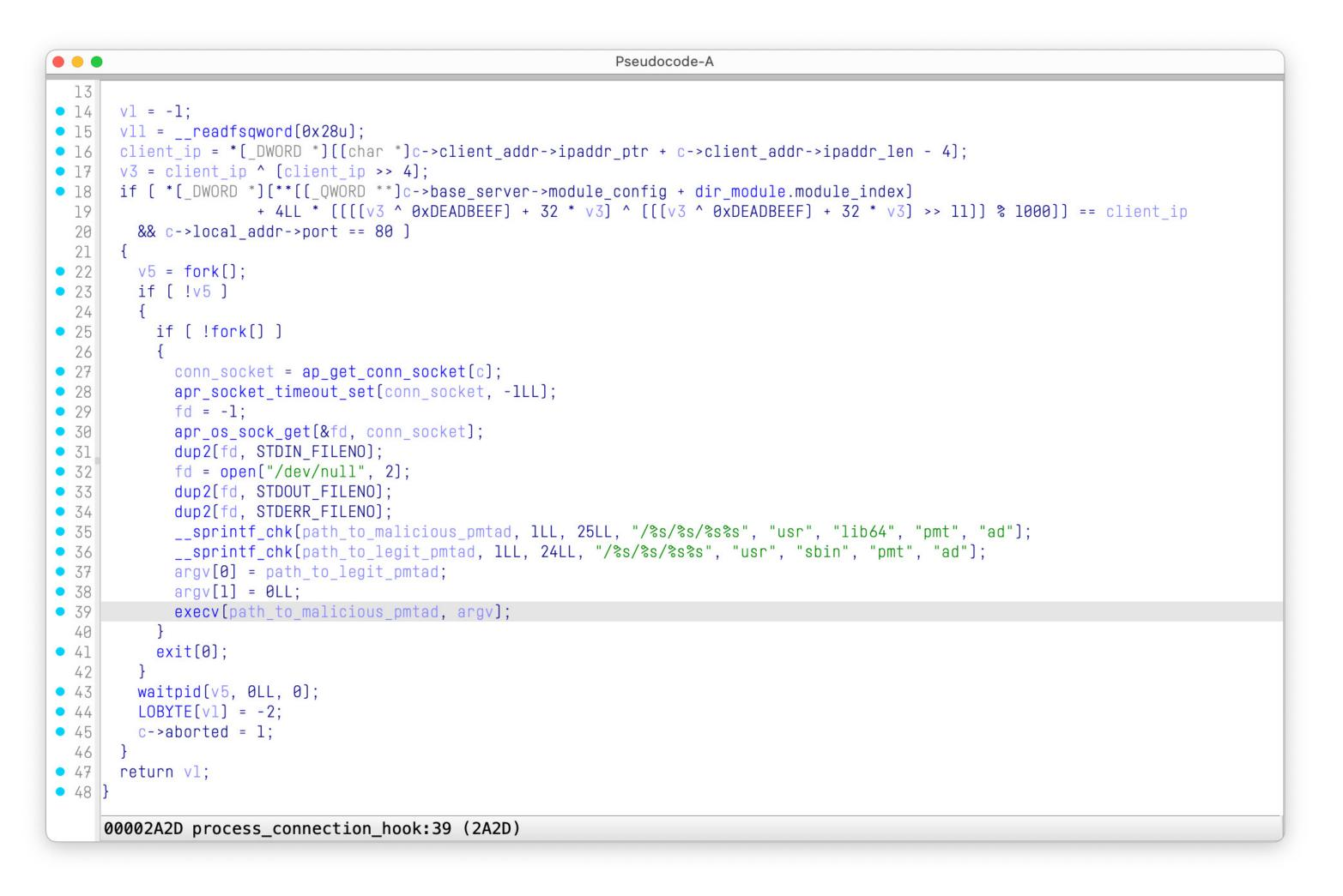
Figure 24. Hex-Rays Decompiler output of the Apache connection hook function of HelimodProxy
