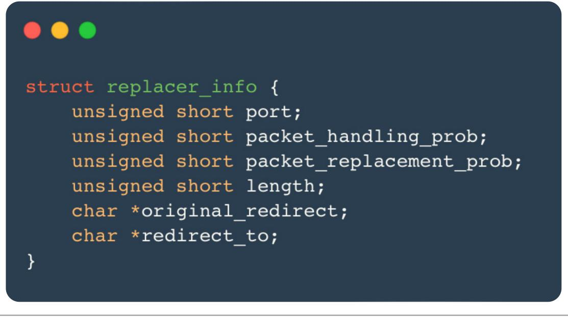
Figure 35. Structure of the hardcoded configuration
