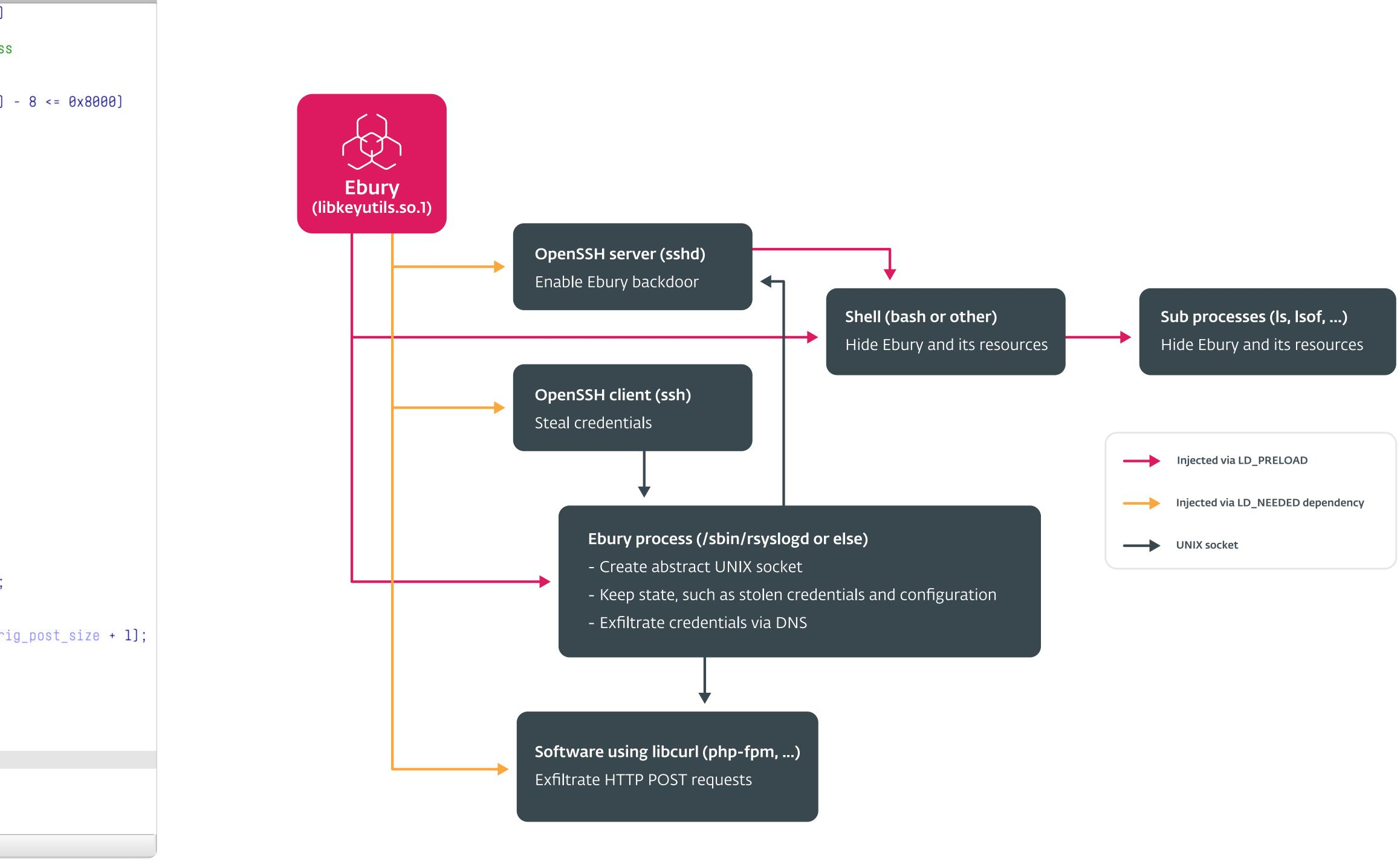
Figure 14. Processes where Ebury is injected
