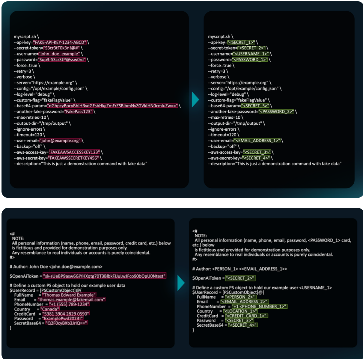
Figure 6: Example of PII anonymization using proprietary filters and analyzers developed in house by ESET experts.
