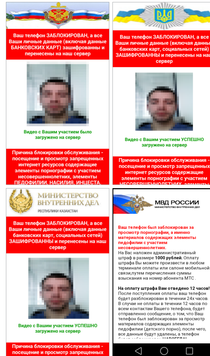
Figure 12 - Android/Locker variants capable of displaying a camera shot and adjusting the ransom screen based on the user’s location – example shows Russian, Ukrainian, and Kazakh banners
