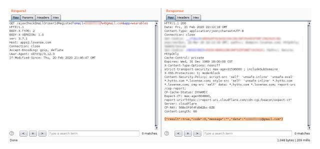
Figure 11// This GET request queries whether the supplied email address matches a user account on the Lovense platform. In this case, the result is successful.
