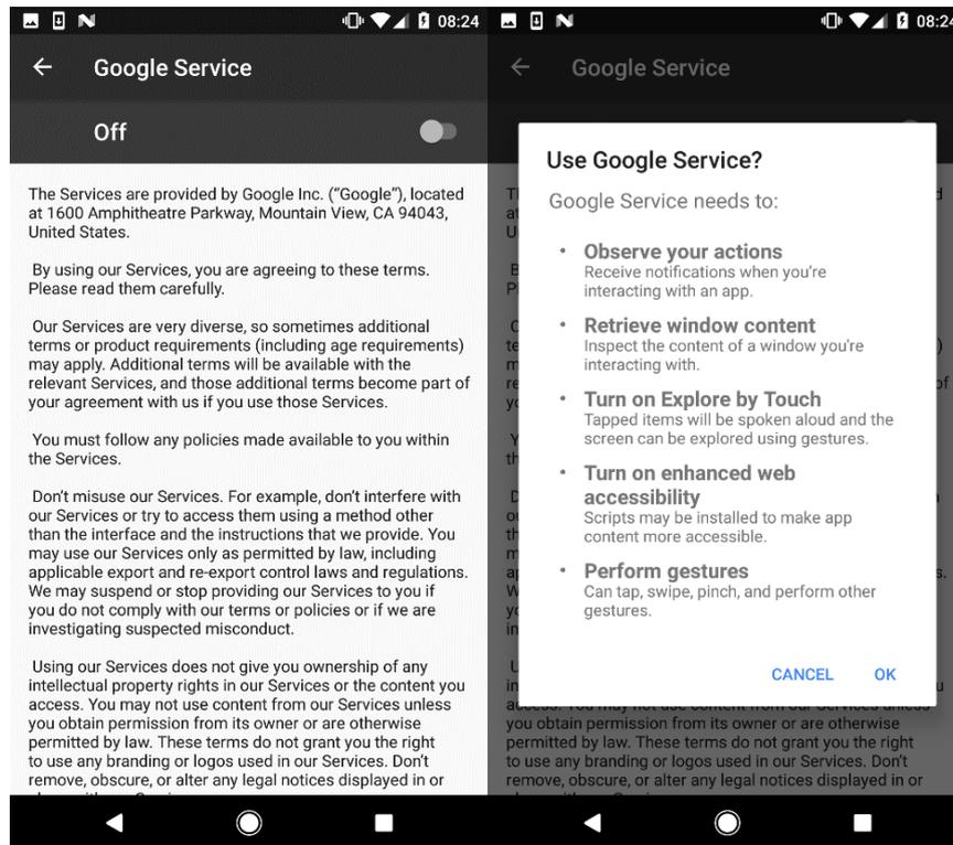
Figure 7 // A variant of BankBot requesting the activation of its malicious Accessibility service disguised as “Google service”, and using a description taken from Google’s original Terms of Service
