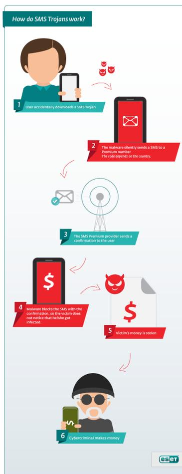
Image 1: How an SMS Trojan operates
